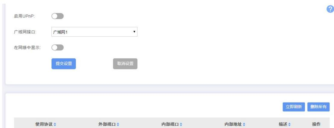
The screenshot shows a configuration panel for UPnP. It includes three settings: '启用UPnP' (Enable UPnP) with a toggle switch, '广域网接口' (WAN Interface) with a dropdown menu set to '广域网1', and '在网络中显示' (Show in network) with a toggle switch. Below these are '提交设置' (Submit settings) and '取消设置' (Cancel settings) buttons. A table below the panel has columns for '使用协议', '外部端口', '内部端口', '内部地址', '描述', and '操作'. There are also '立即刷新' (Refresh immediately) and '删除所有' (Delete all) buttons.
