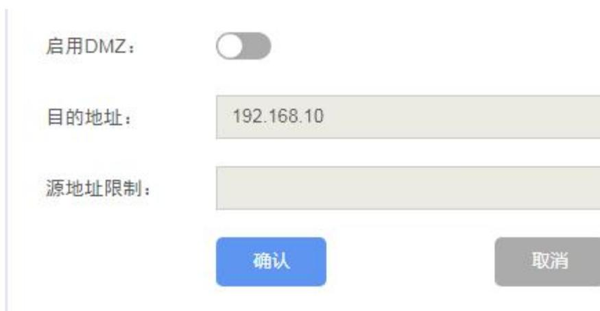
The image shows a DMZ configuration window. It has three main sections: 1. '启用DMZ:' (Enable DMZ) with a toggle switch currently turned off. 2. '目的地址:' (Destination Address) with a text input field containing '192.168.10'. 3. '源地址限制:' (Source Address Restriction) with an empty text input field. At the bottom, there are two buttons: '确认' (Confirm) in blue and '取消' (Cancel) in grey.
